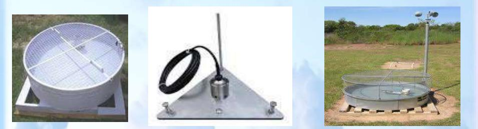
An atmometer or evaporimeter is a scientific instrument used for measuring the rate of water evaporation from a wet surface to the atmosphere. Atmometers are mainly used by farmers and growers to measure evapotranspiration rates of crops at any field location.
