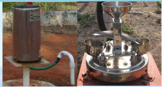
The sensor is the tipping bucket mechanism and is mounted at a height of 0.6 to 1 m. The collector diameter is 20 cm.
