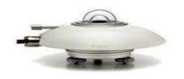
A **pyranometer** is a type of actinometer used for measuring solar irradiance on a planar surface and it is designed to measure the solar radiation flux density (W/m<sup>2</sup>) from the hemisphere above within a wavelength range 0.3  $\mu$ m to 3  $\mu$ m.
